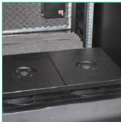
Double cooling system design
